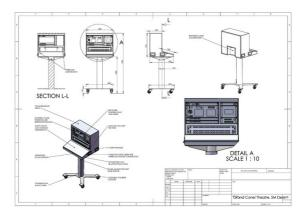
The Wooden enclosure SMConsole offers a large control area and can accommodate up to 24 cue light channels, additional touch panels for working light controls and a further 19" panel section on the right for extra facilities.
