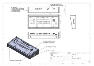
The larger console case can be made any width depending on the facilities that are required. In general the left section is reserved for clocks, timers and intercom, the middle section is cue lights, with functions such as paging and intercom on the right panel.
