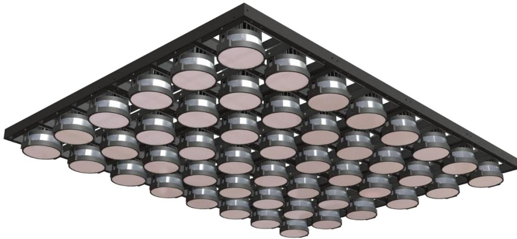
To deliver seamless scalability, the DF System was designed using aircraft aluminium modular frames to contain the LED engines. Configurations of the frame were installed with minimum stress using M10 threaded bars, that could be easily fixed to the existing roof structure.
